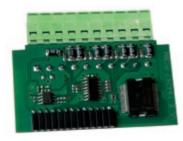
configuration tool (version 4.4 and higher) it is a simple process to choose if a particular I/O will be binary input or binary output.
