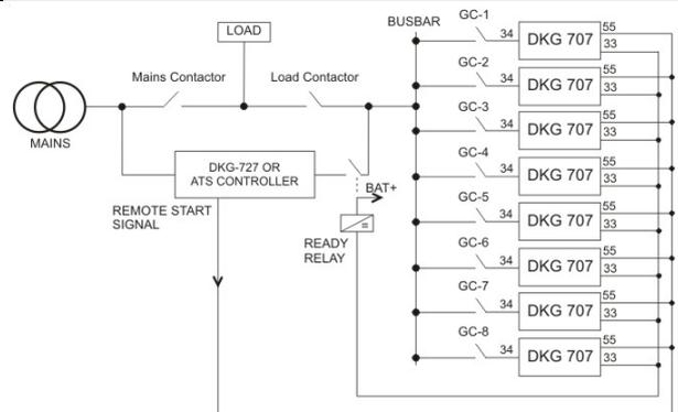
The unit allows the synchronization scheme defined in the above picture. The application is made with standard units and standard software, without extra cost. No additional parts are needed.
